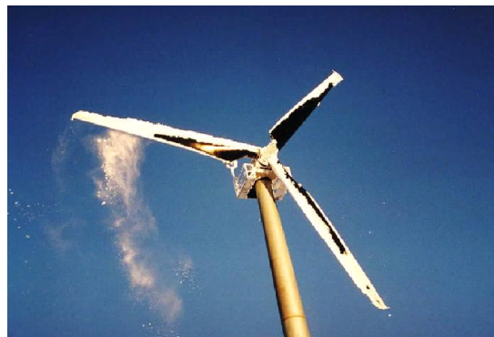
Figure 8.6: Black coated blade with ice shedding [35]
